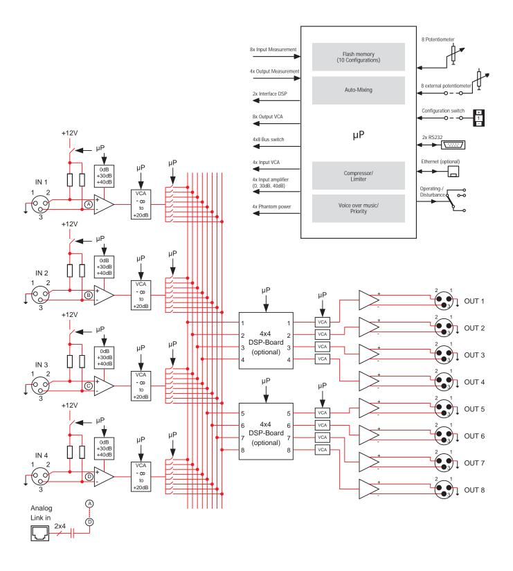
You can optionally add up to two 4x4 DSP matrix modules to your ITEC MULTISPLIT. ITEC SPLITDESIGN includes to configure these DSPs. They operate in 24 Bit / 44,1 kHz mode and provide optimal algorithms. Each DSP has 9 filters per input that can be parameterized. Attenuation, quality and frequency can be adjusted. Each output can be delayed (0.023 – 500 ms) and filtered by setting a high/low-pass filter (1. to 4. order)
